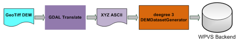
Fig. 8: DEM to deegree3 data conversion toolchain.
